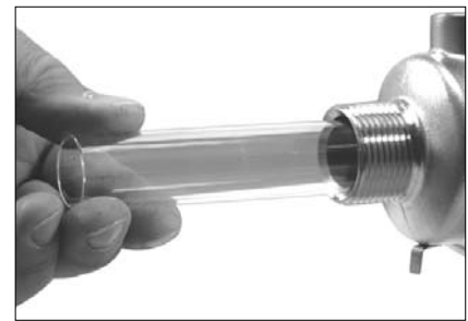
Step 6 - Remove Quartz Sleeve
