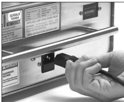
Step 1 - Disconnect Power Cord
