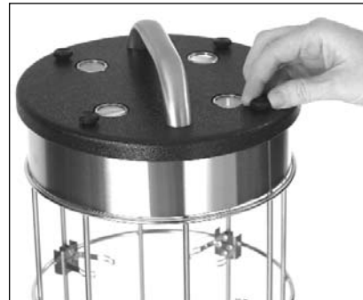
Step 3 - Loosen Four Thumbscrews
