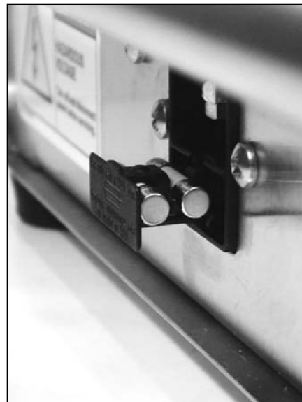
Step 2 - Open Tray (Spare Fuse is Clipped in Front of the Active Fuse)
