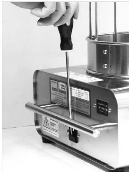
Step 1 - Insert Screwdriver & Bring Tray Forward
