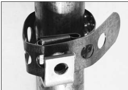
Step 1 - Wrap Strap Tight Around Pipe
